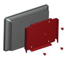
Mount the display bracket to the back of the rear facing display using the 75mm x 75mm VESA mounting holes
