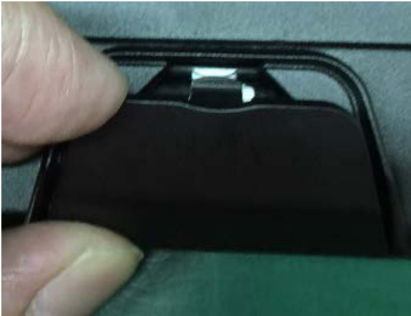
1. Remove the Barcode cover
