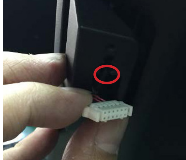
2. Install MSR holder with 2 screws
