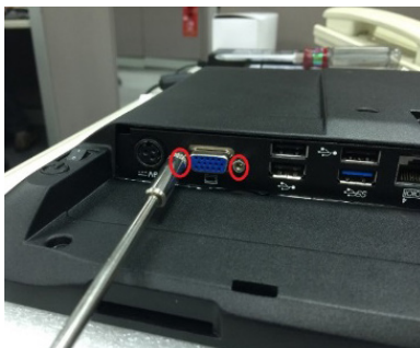
7. Unscrew 2 screws on VGA
