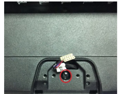
6. Unscrew 1 screw on Barcode
