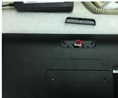
5. Unscrew 1 screw on VFD
