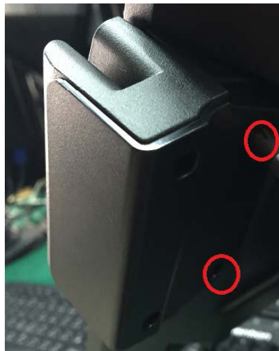
4. Install MSR with 2 screws
