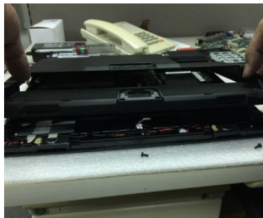
8. Remove the back cover
