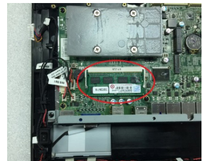
9. Put the memory into socket
