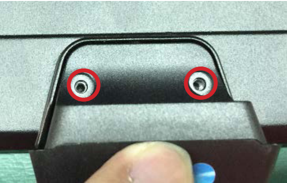
3. Install Barcode with 2 screws
