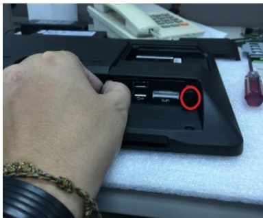
4. Unscrew 2 screws I/O Board
